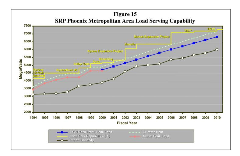
Without the Palo Verde to Southwest Valley 500 kV line in 2003, APS peak load serving capability would be inadequate until construction of the Trilby Wash to El Sol 230 kV line in 2006. Similarly, without the Palo Verde to Southwest Valley 500 kV line in 2003 and the 575 MW reduction of the Kyrene plant expansion in 2002, SRP's load serving capability would be inadequate to meet its peak load obligations until the Santan plant expansion in 2006.
