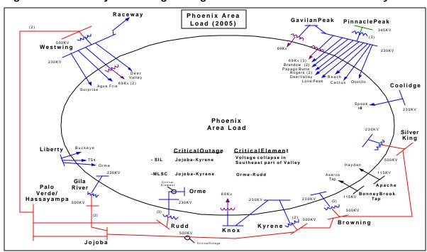
Figure 21: New Projects Strengthening the Phoenix-Area Transmission System
