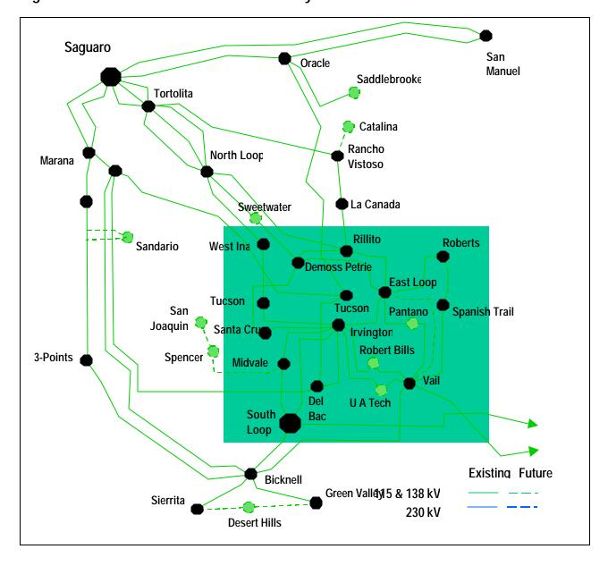
Figure 17: Tucson Area HV Transmission System
