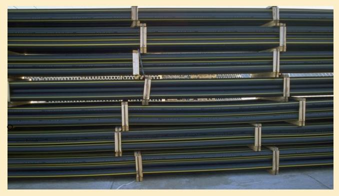
PE 4710 ASTM - D2513 4" Diameter, SDR = 11 Ambient Temp. 84° F
