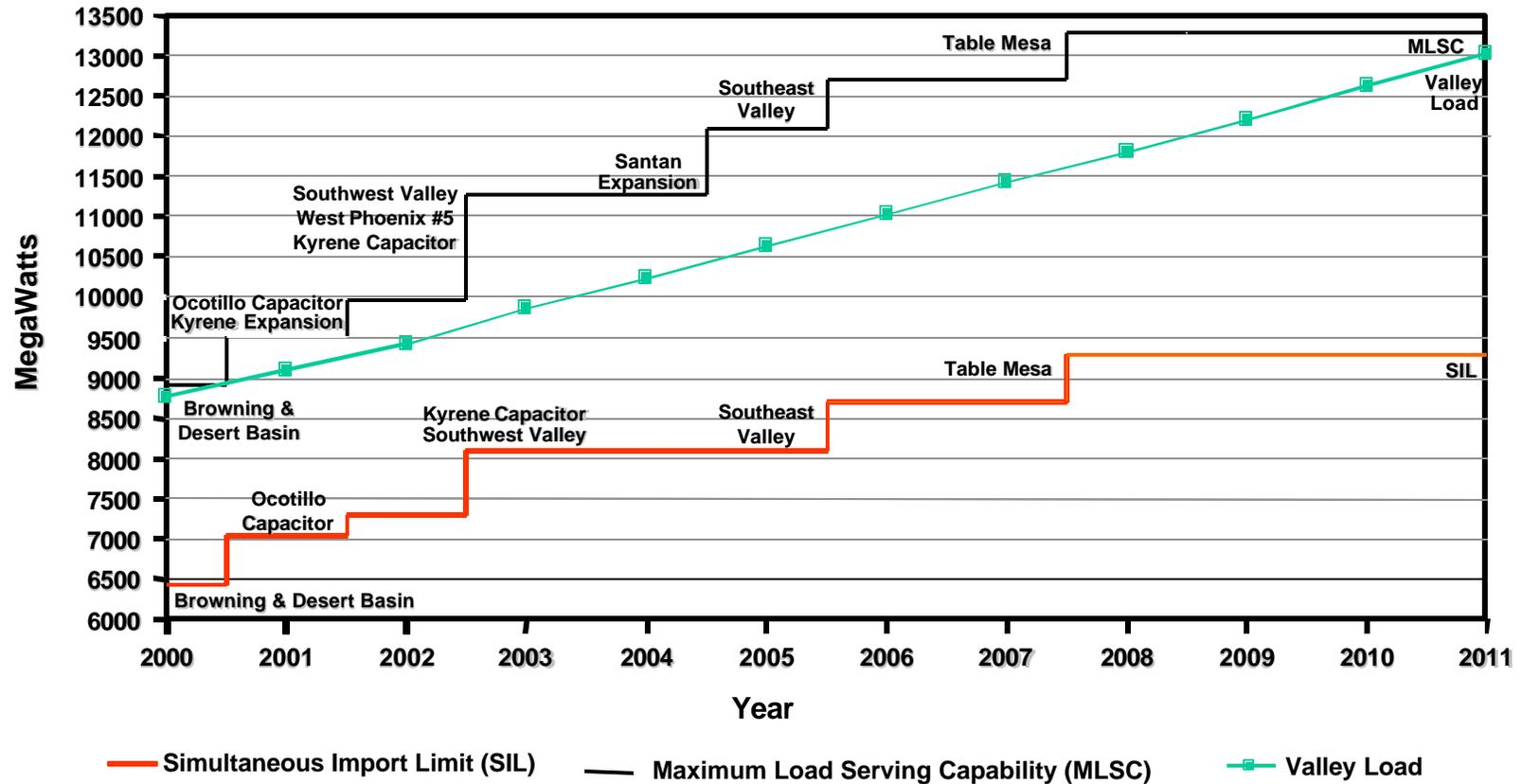
The nomogram depicts the effects of transmission line additions or upgrades on import capability and the voltage constraints while taking into account all the capacitor and transmission system additions that are shown in Figure 7.4. Through the (N-1) contingency analysis, APS and SRP found the most limiting contingency that drives the Mvar margin. It is a Palo Verde (Jojoba) to Kyrene 500 kV line outage for which the Kyrene 230 kV substation is the most limiting Mvar margin bus.
